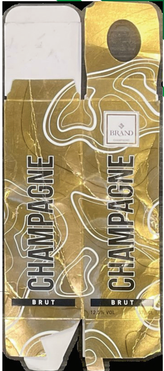
Figure 2 captures the total image of one of the most densely covered test pieces, the Champagne folding carton, V2. It is an example of one of the eight products tested and had an estimated 75% metallic decoration coverage. The test results proved it to be 100% sortable.
